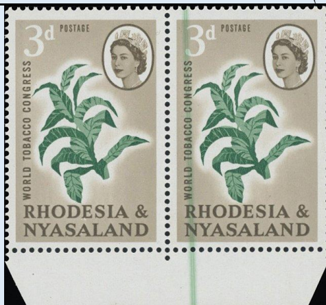
Vertical doctor blade flaw (Source rhodesia.co.za)
