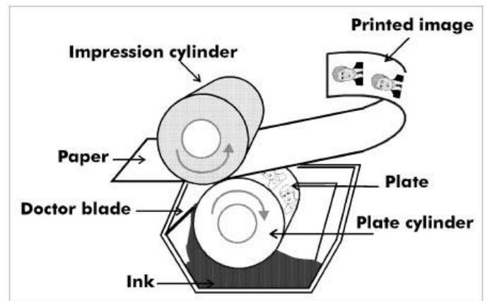
The single unit of the printing press is one of several units linked together to give a continuous print run. Below is a diagram of a seven unit press, which is more common today than it may have been in the 1960's. By having several colours in a print run, the quality of the printing can be improved considerably.
